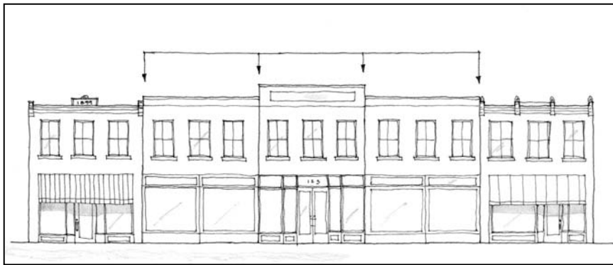
Large new buildings should be designed with vertical divisions to be consistent with traditional historic building widths.
